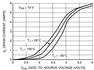
Figure 2. Transfer Characteristics
