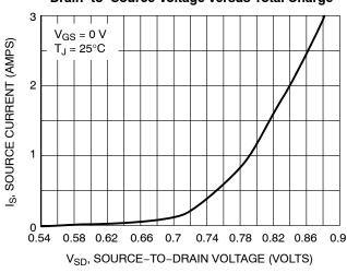
Figure 10. Diode Forward Voltage versus Current
