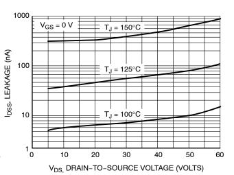
Figure 6. Drain-to-Source Leakage Current versus Voltage
